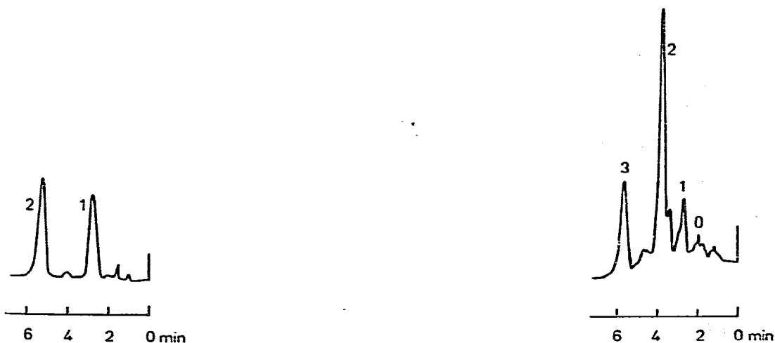
Fig. 6. Separation of oligomers Z-Glu(DIME)-OBzl (1) and Z-[Glu(DIME)] 2 -OBzl (2). Packing: ODS-TMS silica, eluent: methanol-water-acetonitrile (5:4:11, v/v/v); sample: 5 \mu g of each oligomer; flow-rate: 1.3 cm 3 /min; detection: 254 nm; 0.05 a.u.f.s.
